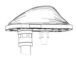
When mounting the antenna on a bracket, an additional cable protection kit can be used. Our conduit support kit (Art. no. 84079593) allows the use of standard M40x1.5 conduit guides. Please refer to the mounting instruction of article 84079593.
